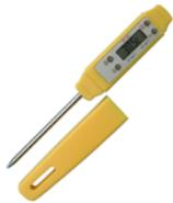
with baby dials making it easier when measuring thin items. Regardless of the thermometer sensor depth, it is still important to measure the temperature at the thickest part of the item you are testing. The average cost of a digital is around \$10-\$20.
